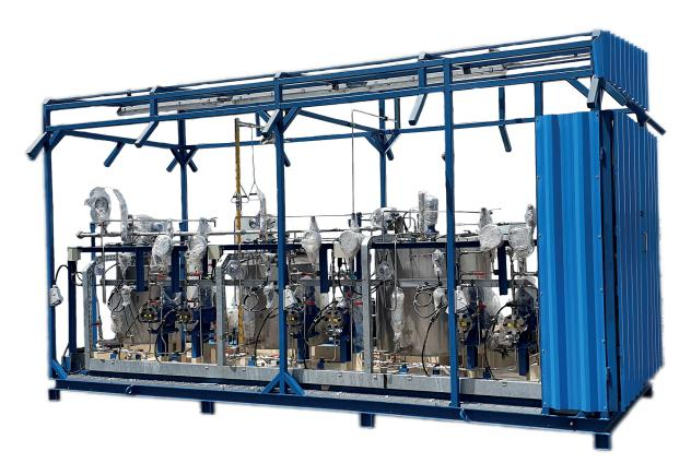
Chemical Injection Skids (CIS) is an integrated system used to dose and inject various chemicals into different pipelines at various conditions. In the Oil and Gas industry this helps to increase production, reduce corrosion and to improve the process. High level of accuracy is required for dosing system because of the environmental and financial reasons. Based on the flow/pressure requirements and various chemicals used, the metallurgy and the design of the skid changes.
